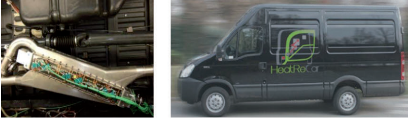
Fig. 10. Left HEATRECAR prototype TEG. Right Iveco Daily integrating the TEG.
