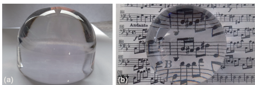
Fig. 5. Modern reconstruction, for the author, of a medieval reading stone by Colin Rennie, University of Sunderland. (a) Glass cylinder with end section which is a part of a hemisphere. (b) Magnification of text when the reading stone is slid over the page.
